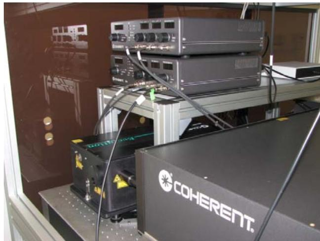
Figure 3.3. Evolution Nd:YVO laser system provides pumping energy at its second harmonic for regenerative amplifier (Legend). The system is controlled using a notebook through two control boxes visible in the upper part of the picture.
