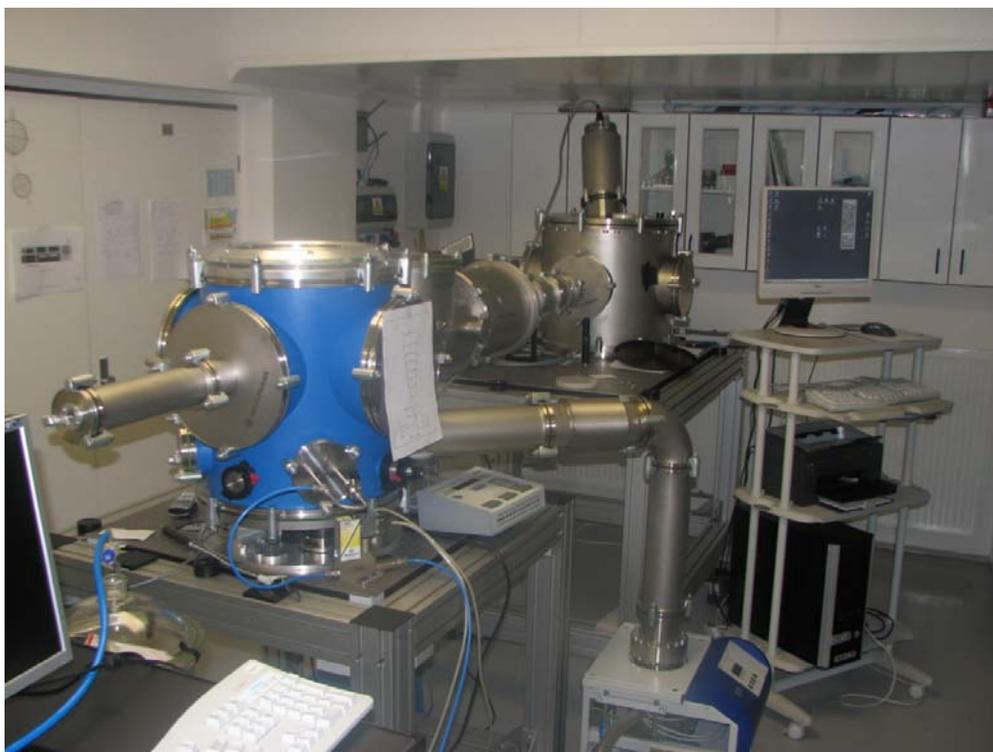
Figure 3.5. HHG experimental beamline at IoP/PALS. The beamline comprises titanium-doped sapphire laser system, HHG source placed in the source vacuum chamber (the blue in the picture) and application chamber (grey in the picture, downstream beam propagation direction).
