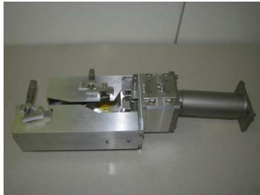
Figure 3.10. Real photo of TGS (the CCD portal is at the right hand side of the spectrometer in the photo).
