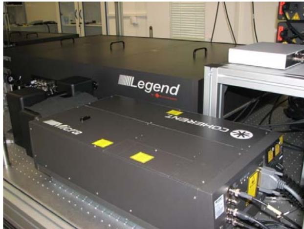
Figure 3.2. Picture showing the table-top femtosecond laser system deployed in the HHG source. The system comprises Micra oscillator and Legend regenerative amplifier pumped by Evolution laser (visible in Figure 3.3).
