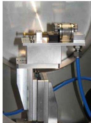
Figure 3.7. Picture of the gas cell used in the experiments.
