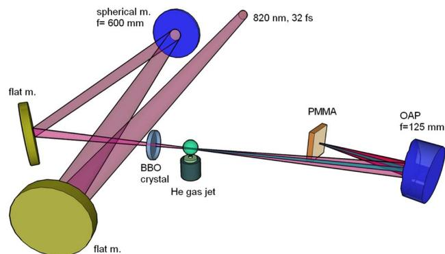
FIG. 1. (Color online) Schematic of the experimental setup for surface modification by dual action of XUV and visible-NIR ultrashort pulses.
